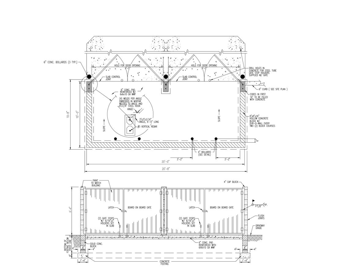
**PROP. 10'X20' MASONRY TRASH ENCLOSURE DETAIL**
