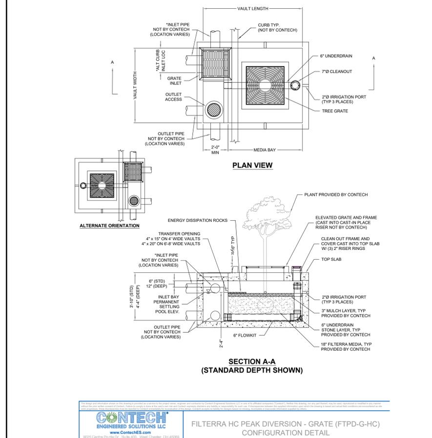
**FILTERRA TREATMENT DEVICE DETAIL**
